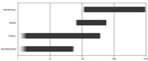
Figure 5. Approximate Liquid Chiller Availability Range by Compressor Type
