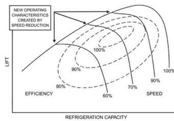
Figure 10. Typical Variable-Speed Centrifugal Compressor Performance (Carrier 2004)
