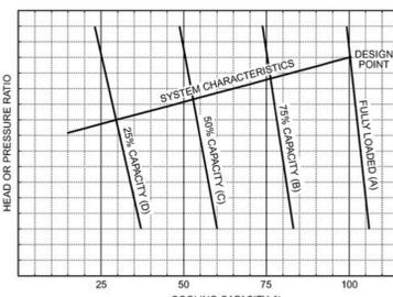
Figure 7. Reciprocating Liquid Chiller Performance with Three Equal Steps of Unloading
