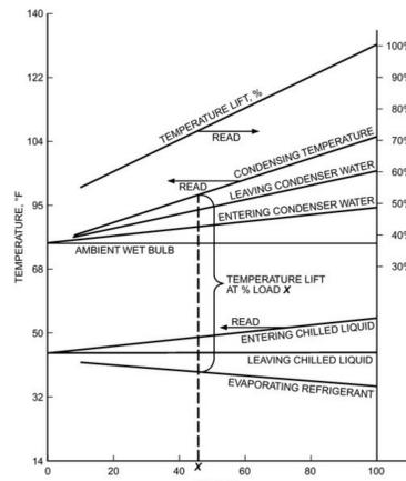
Figure 11. Temperature Relations in a Typical Centrifugal Liquid Chiller
