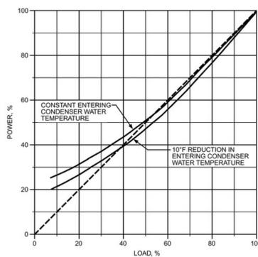
Figure 13. Typical Screw Compressor Chiller Part-Load Power Consumption
