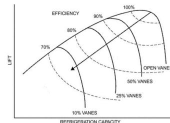
Figure 9. Typical Centrifugal Compressor Performance at Constant Speed (Carrier 2004)
