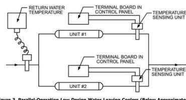
Figure 3. Parallel-Operation Low Design Water Leaving Coolers (Below Approximately 45°F)
