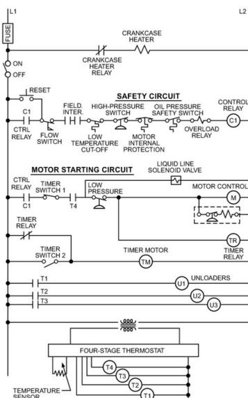
Figure 8. Reciprocating Liquid Chiller Control System
