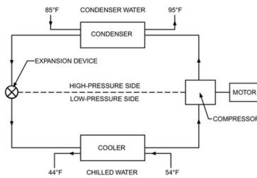
Figure 1. Equipment Diagram for Basic Liquid Chiller
