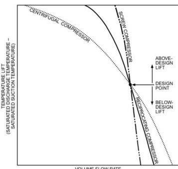
Figure 6. Comparison of Single-Stage Centrifugal, Reciprocating, and Screw Compressor Performance
