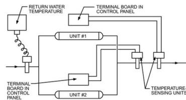
Figure 2. Parallel-Operation High Design Water Leaving Coolers (Approximately 45°F and Above)
