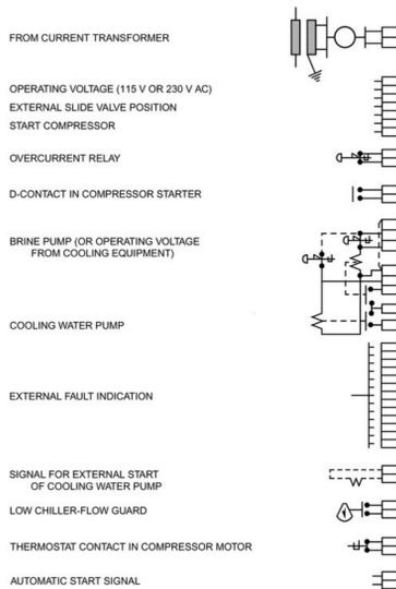
Figure 14. Typical External Connections for Screw Compressor Chiller
