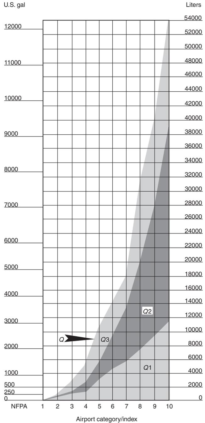
FIGURE B.6 Comparison of Water by Volume of  $Q_1$ ,  $Q_2$ ,  $Q_3$ , and  $Q$  for Producing Foam Solution Using AFFF.
